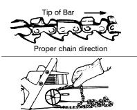
Place chain onto the sprocket
